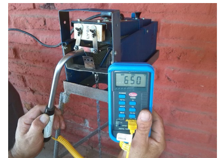
Pyrometer indicating proper blade temperature of 650°C.
